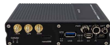
PL-R5 BASIC M2 IP20 [Standard Type] M.2 slots ×2 Supports simultaneous LTE and Hailo implementation
